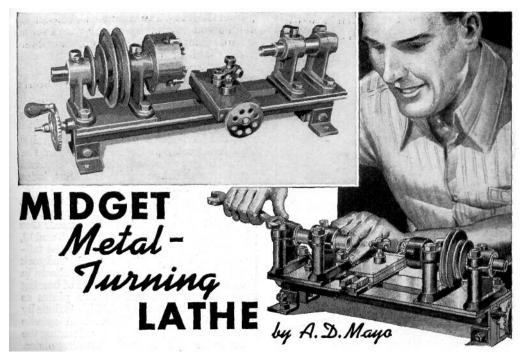
RAFTSMEN, modelmakers and others who need a small metal-turning lathe can make one almost entirely from scrap material available in junk or auto-wreck-ing yards. A chuck may have to be purchased, but many turning jobs can be done between centers or on an improvised face-plate. The lathe shown here has a swing of 41/2 in. A larger one, of course, can be made by changing the proportions. In. making the ways, Fig. 1, select straight
