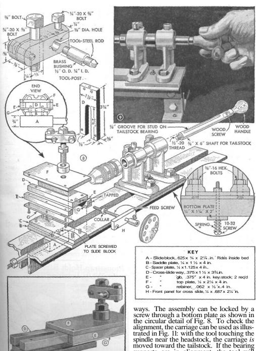
supports are in alignment, the tool will touch the spindle uniformly throughout its travel from end to end.
